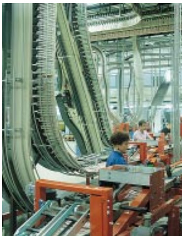
Tampereen Kirjapaino Oy's Postpress Unit can add up to four separate inserts in the main product.
