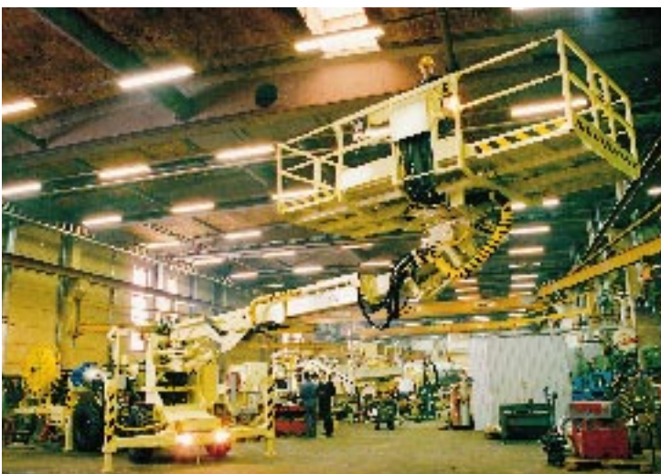
HIMEC 9910 B HEX is a lifting platform vehicle for large-scale tunnel support and installation work. The vehicle, with its turning and hydraulically expanding working platform, is designed to meet the special needs of customers.
