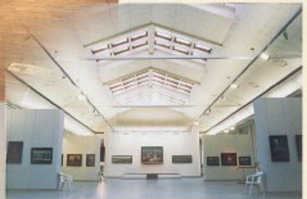
The daylight dependent lighting control system in Moscow's exhibition centre, Little Manege, uses Helvar FD dimmable electronic ballasts.
