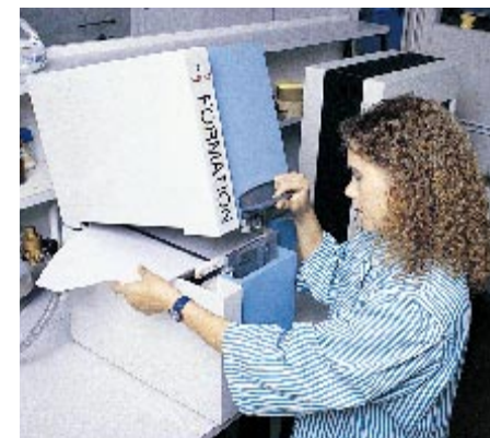
The new Kajaani formation analyzer improves measurement accuracy and repeatability compared to conventional visual assessments of paper samples. It can be easily used to test individual sheets or for the fully-automated testing of paper profiles.
