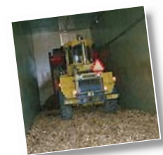
The material to be composted is in the tunnel for a period of one to two weeks, after which it is allowed to mature.
