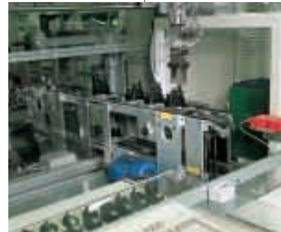
THE PNEUMATIC GRIPPER PICKS THE COMPLETED PRODUCTS UP OFF THE BELT, AND THE EMPTY ASSEMBLY PALLET THEN RETURNS ALONG THE LOWER TRACK TO THE FRONT END OF THE PRODUCTION LINE.
