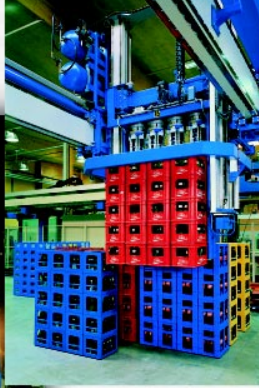
Cimcorp Oy delivered a loading gripper for a pick-up system to Oy Hartwall Ab's factory in Lahti. The gripper's air processing units and rodless cylinders were supplied by IMI Norgren Ltd.
