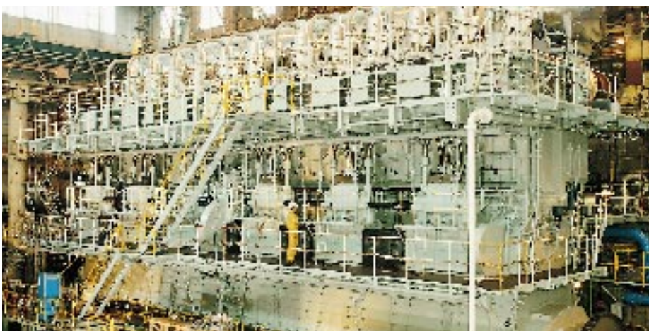
The Wärtsilä 64 engine for power plants and marine applications is the largest medium-speed engine in the world. Shown here is the exhaust manifold being assembled.
