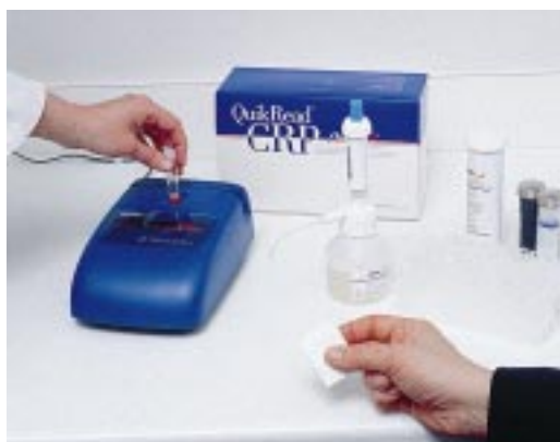
The new QuikRead is a rapid quantitative method for measuring CRP from whole blood. The system is easy to use and it gives the results in less than four minutes.
