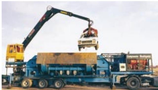
**Loglift and Jonsered are Europe's leading forestry crane brands but are also used in a wide variety of other applications, i.e. handling scrap, waste and recycling. The cranes' power and performance make them suitable for both mobile installations or stationary mountings at sawmills, recycling depots, docks etc.**
