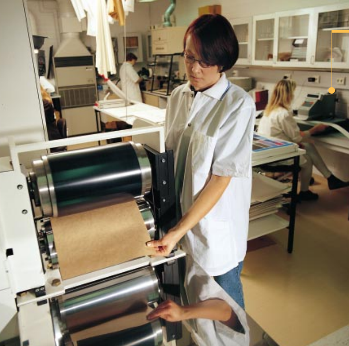
A laboratory calender is used to simulate the polish and smoothness of paper in production. Laboratory worker Eveliina Hopeanala at work.
