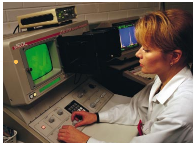
Laboratory worker Virpi Tuominen using an electron microscope (SEM/EDXRF) to examine the paper surface.
