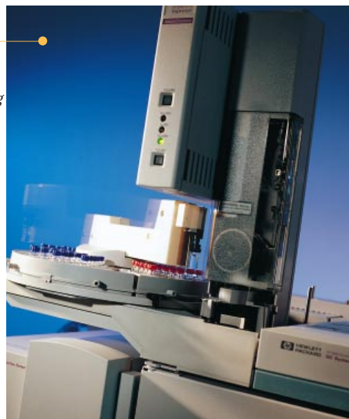
An automatic sampler in a combined gas chromatograph and mass spectrometer used for analysing the structure of various compounds and identifying sterols.
