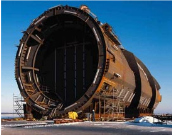
TM steels developed by Rautaruukki are finding a growing number of applications in demanding bridge and offshore projects. A new alternative that is being studied is the use of titanium in the killing of thermomechanically manufactured steels.
