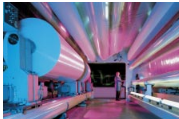
Atlas' 9.5 meter wide slitter rewinder, designed for film, is one of the Converting Equipment Group's most successful products.
