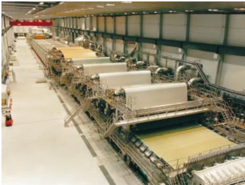
The world's largest board machine, containing much of Valmet's latest technology, such as a four-station on-machine coater, was delivered to Stora Skoghall in Sweden for the production of liquid packaging board.
