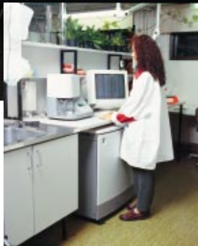
Kajaani FiberLab offers unique exact measurement of fiber length and, as new features, fiber width and cell wall thickness measurement.
