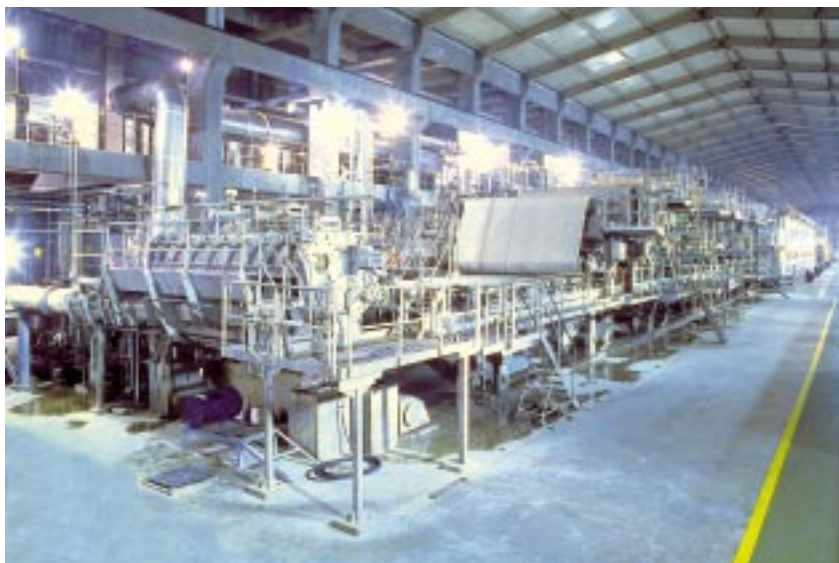
The testliner and corrugating medium board machine delivered to the South Korean company, Asia Paper, has the country's first shoe press on a board machine.
