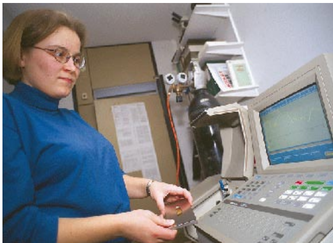
Minna Salonen uses an FTIR spectrometer to study the properties of compost.
