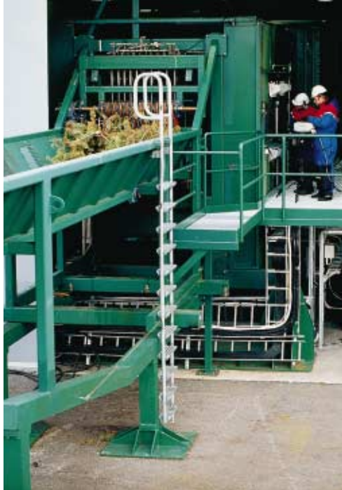
The research equipment for whole-tree processing supports the development of new delimiting, debarking, chipping and screening methods.
