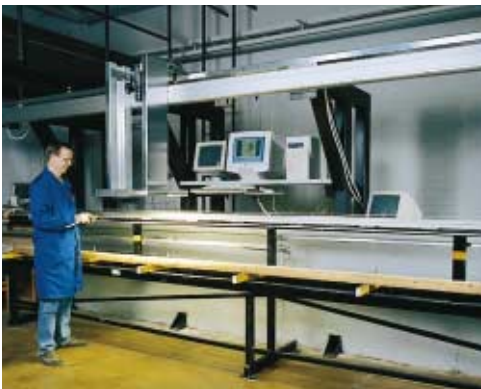
A machine vision system based on a colour camera is being used in the modelling of the raw material of the mechanical forest industry.
