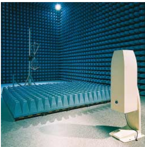
The EMC laboratory serves the electronics industry by testing the electromagnetic radiation of equipment.
