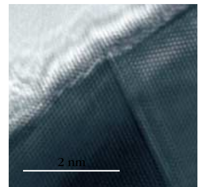
High resolution transmission electron microscope image of silver particle surface.
