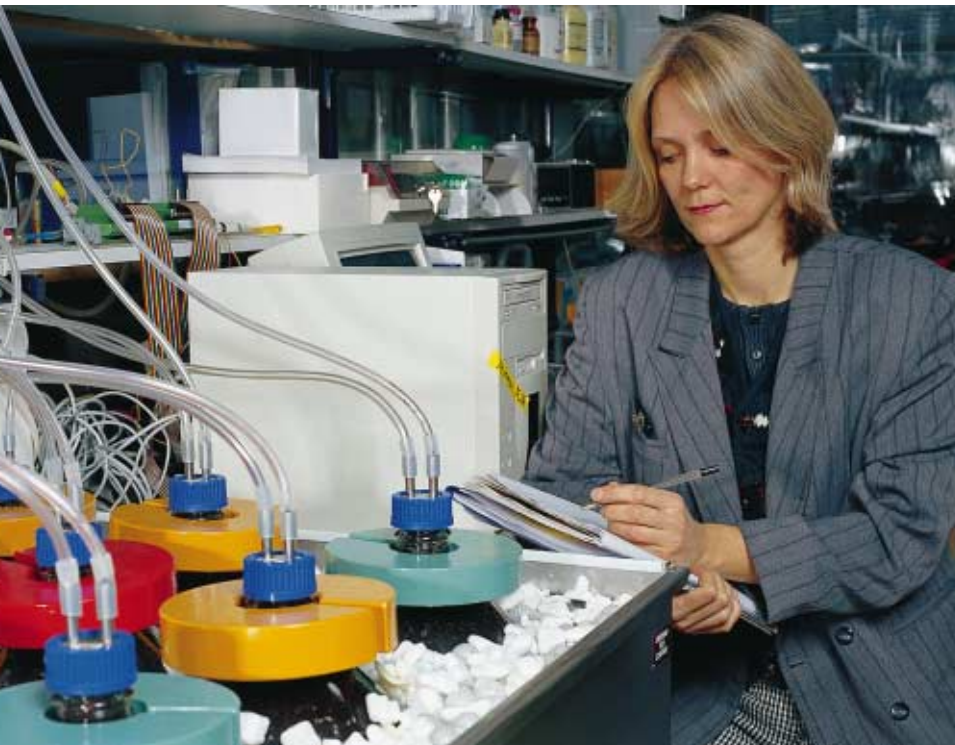
The biogradability of packaging materials is studied in controlled composting conditions.
