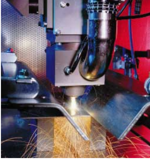
Finland's first high-energy Nd:YAG laser enables VTT to transfer new technology for metal workshops.
