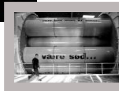
Örtofta Sugar Factory is one of Danisco Sugar AB's four factories in Sweden. The picture to the right from Danisco Sugar's Nakskov Sugar Factory shows the drum in which the sugar is dried at one of the final stages of the process.
