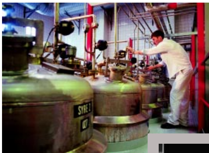
Danisco Ingredients' plant at Grindsted in Denmark produces enzymes by fermentation in large closed tanks. The gloves on the shelves are part of the employees' protective clothing.
