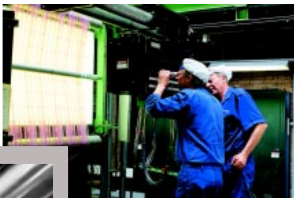
Production at Danisco Flexible Raackmann's Horsens site in Denmark is being monitored around the clock. Here two employees are keeping a watchful eye on the printing quality of the packaging. The small picture shows a gravure printing cylinder.
