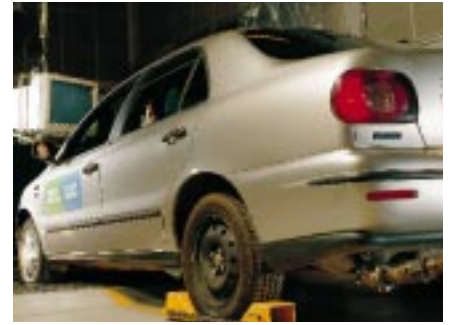
In Kemira Metalkat's laboratory, tests are being carried out on an exhaust gas catalytic converter that is suitable for use in a vehicle that runs on two alternative fuels: natural gas and gasoline. (Photograph: Studio Karl Labti)
