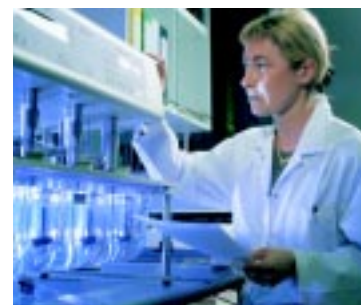
Monica Hildén working with a system used for analysing the dissolution of active substances in orally administered pharmaceutical preparations.
