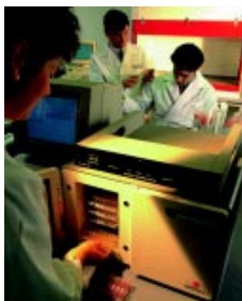
The VITEK system by BioMérieux enables rapid identification of microbes.
