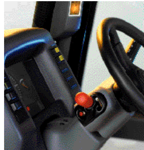
The computer-controlled HiTech forward/reverse shuttle is an example of Valtra's customer-responsive product development. The driver selects the direction with the joystick.
