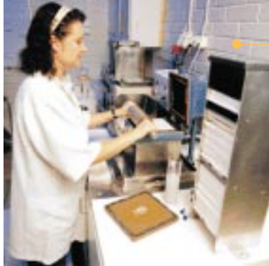
Laboratory worker Hanna Sipilä making test board to be used for studying bonding and how chemicals bind to fibre.
