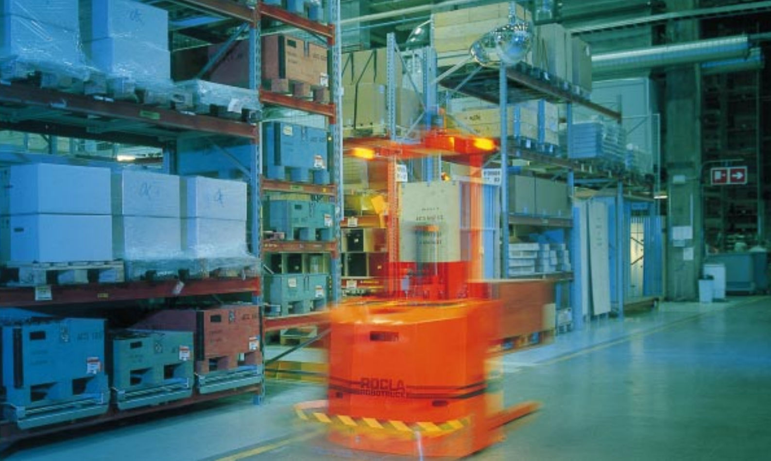
Regular transfers of pallets can be performed by automated fork lift trucks operated by laser navigation (picture: ABB-Drives, Helsinki, Finland).
