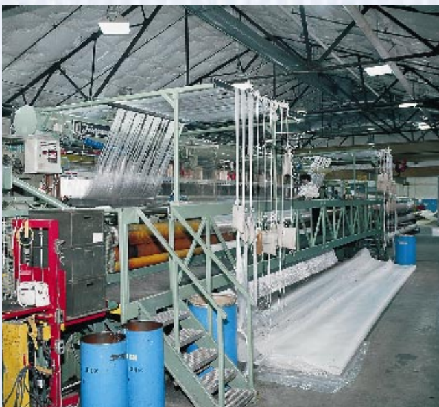
A weaving loom at Canton, rebuilt for the production of the newest styles of seamed press felts.
