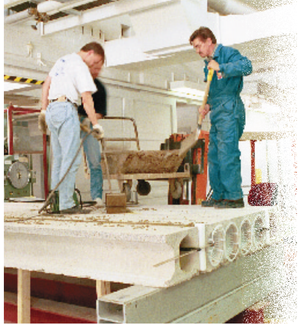
Prestressed hollow-core slabs is the main product of the Group. During 1999 the total production of this product amounted to 7.2 million m 2 .
