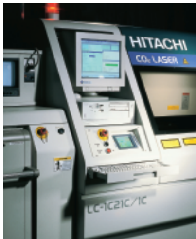
Laser drilling machine for HDI products.
