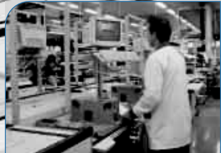
The FPS unit developed for Vaasa Control Oy a production system for the manufacture of frequency meters, on which the products are made from the component stage to despatch.
