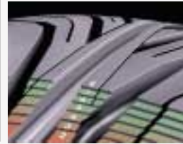
The number on the DSI wear indicator shows the groove depth in millimetres. The numbers wear off one by one as the tyre wears.
