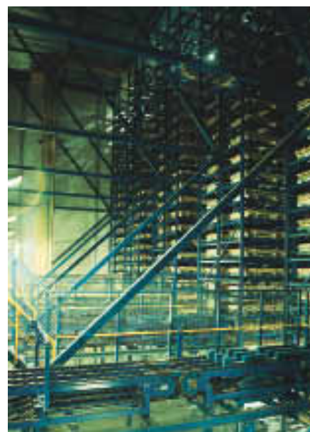
The automated storage facility built in connection with the expansion completed in 1998 can hold up to 11 000 steel pallets ready for loading and delivery to clients.
