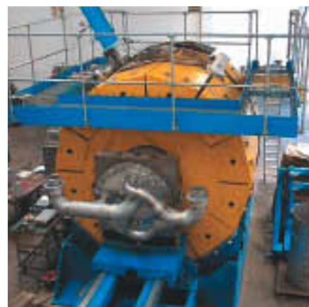
Outokumpu Technology's product range was broadened by acquiring Carpco Inc.'s magnetic separation systems. Pictured is Cryofilter which is based on super-conducting magnetic separation.
