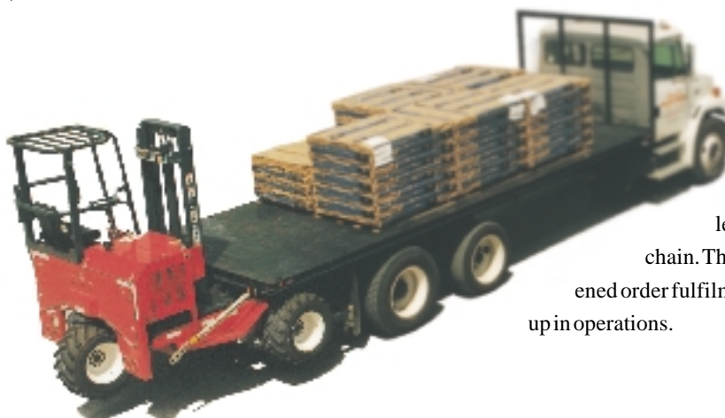
A simple mounting system enables the Moffett Mounty to be secured safely to trucks or trailers without any loss of load space.
