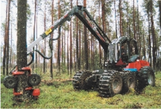
Valmet 921 is the giant in Partek Forest's Harvester program. Since 1999 it can be equipped not only with a telescopic crane, but also with a parallel crane.
