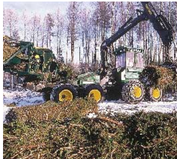
Wood will constitute more than half of the fuel for the world's largest biofuel power plant currently under construction in Pietarsaari in western Finland. Annual fuel consumption will be about 3.5 TWh. Wood residue from logging will be packaged into bales. The energy content of a single bale of 0.6 cubic metres is about 1.1 MWh. The following have a corresponding energy content: - 1.2 cubic metres of peat, - 160 kg of coal, - 100 kg of heavy fuel oil, - 1100 cubic metres of birch wood trunks, - 3.7 grams of uranium.
