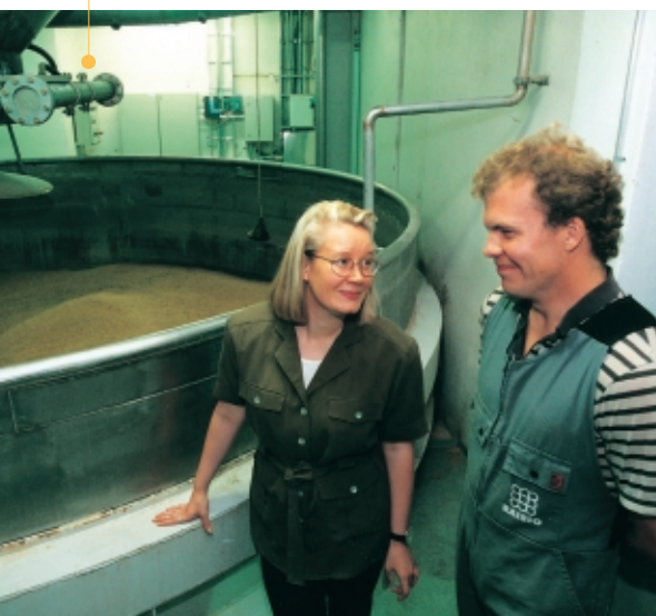
Malting Subdivision process development engineer Riina Pohjolainen and maltster Hannu Koivisto, at one of the Raisio malting plant's fifteen steeping tanks which process altogether 240,000 kilos of barley a day.
