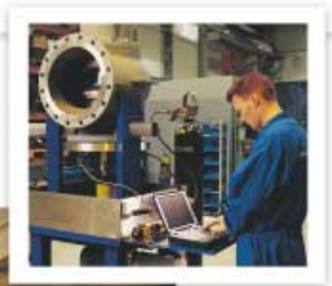
Testing and verification of index values of safety valves in the Hakkila assembly centre.
