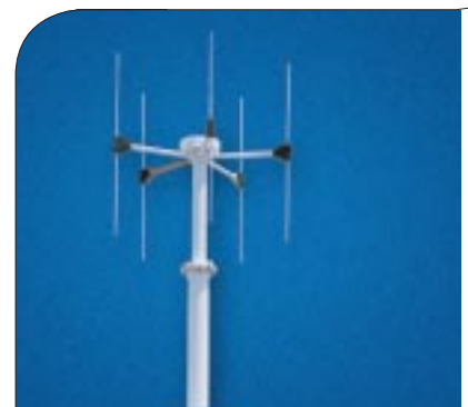
The SAFIR System offers complete information on thunderstorms, accurately localizing and characterizing lightning strikes.
