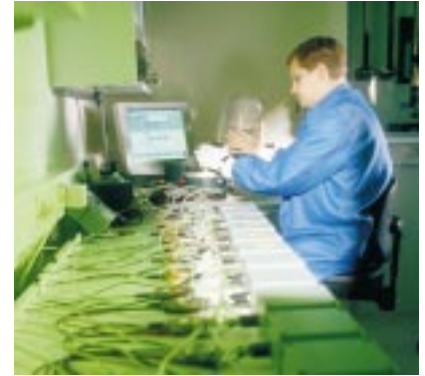
In order to achieve the best possible measurement accuracy, the barometers are calibrated against an accurate death weight tester.
