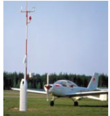
The Vaisala Aviation Weather Reporter is a compact weather observation and reporting system for aviation use.
