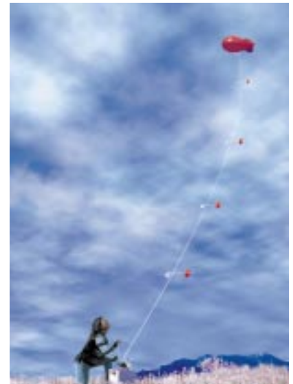
The Vaisala TMT System measures the atmospheric boundary layer.
