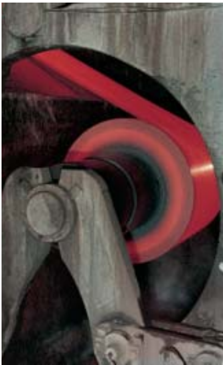
The strip is then coiled before being transferred to the cold rolling mill.
