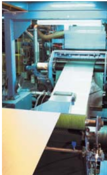
After an initial annealing process, the hot rolled coil undergoes cold rolling and final annealing. During this stage of production, the steel can be rolled to very thin gauges.
