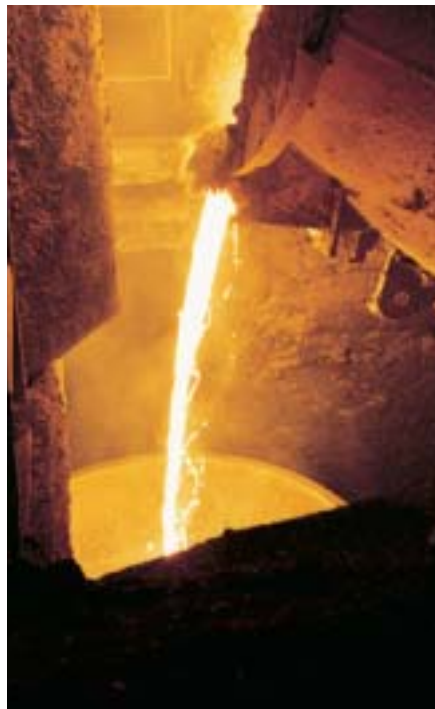
The scrap is melted and alloying elements, such as nickel, molybdenum and chromium, are added.
