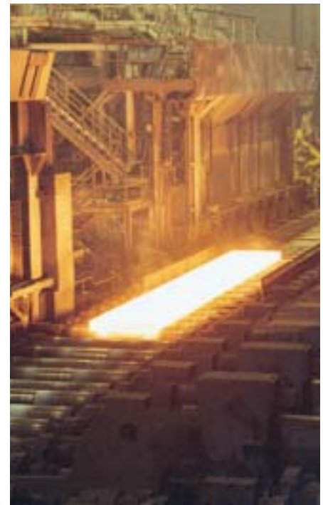
The cast steel slab is rolled to a length of up to one kilometre and down to thicknesses of 2-12 millimetres on the hot rolling mill.
