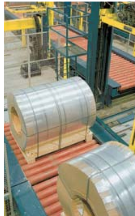
Stainless steel coil products are cut and slit to a variety of dimensions, depending on the intended area of application.
