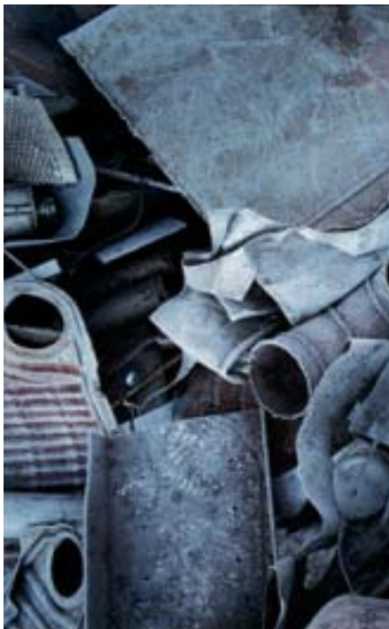
Scrap is the main raw material used in the production of stainless steel.
