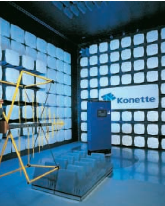
Complete measurements of the electromagnetic compatibility of machines and equipment can be carried out at the EMC laboratory.
