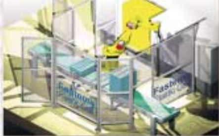
Fanuc injection moulding machine and robotized palletizing system.
