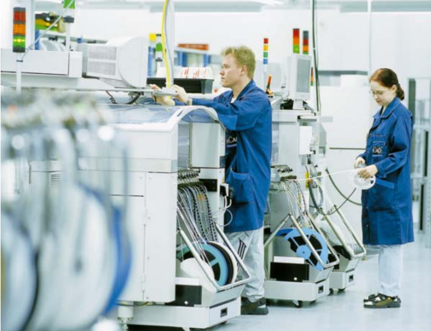
Incap's assembly lines are suitable for both small and large series. The Vuokatti Unit has fast lines for automatic SMD assembly in large series.
