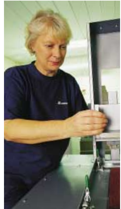
Laboratory technician Airi Leikas tests the chippings of a bituminous sheet membrane in the Company's Central Laboratory.
