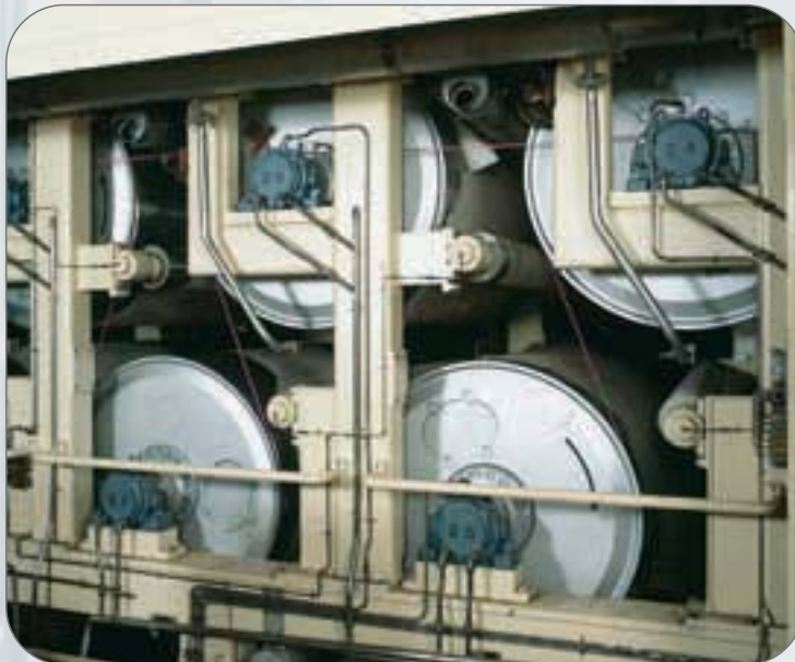
Vahto Oy supplied several drying section rebuilds equipped with drying cylinders.
