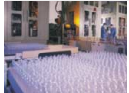
Plastic drying before molding is a common application for dewpoint measurement. Excess moisture in the molding process can cause imperfections in the end products.
