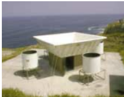
The Vaisala LAP ® -3000 Lower Atmosphere Profiler is a Doppler radar. When combined with a Radio Acoustic Sounding System (RASS) it provides vertical profiles of horizontal wind speed and direction, and vertical wind velocity to an altitude of 3 km.
