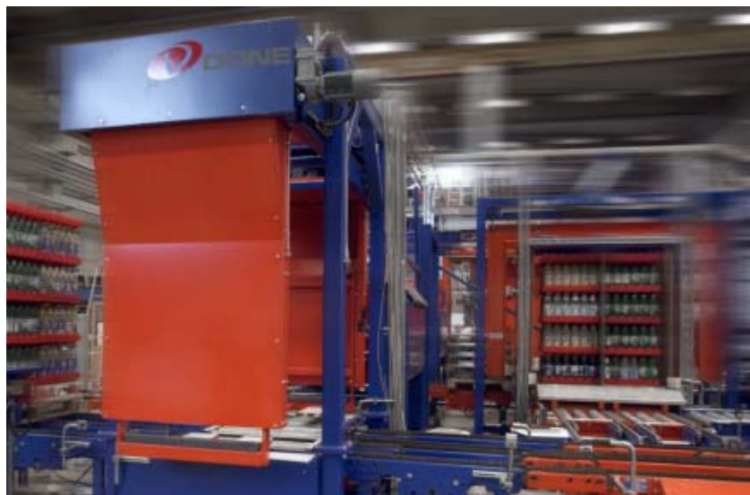
Feed end within the Logistics Systems order-picking system.
