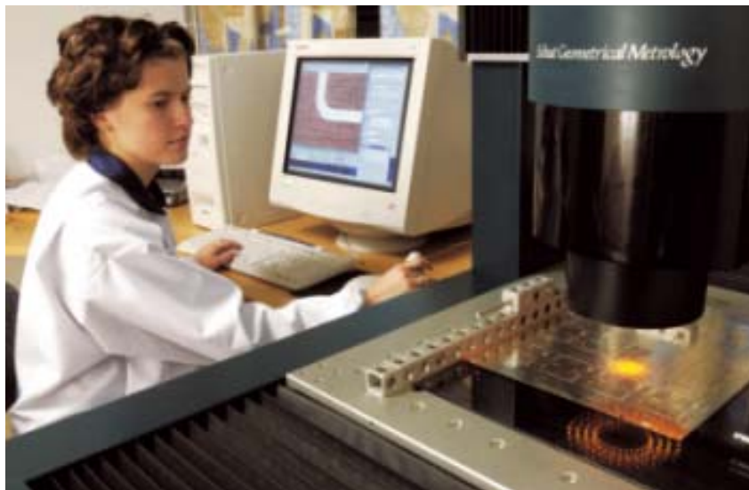
Quality inspection of chemically-milled sheet metal products is performed using optical 2D measuring equipment.
