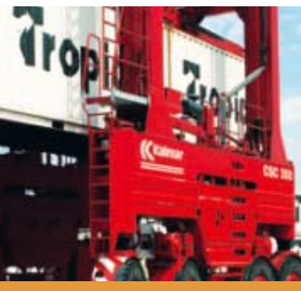
The 15 meter high Kalmar straddle carrier can stack containers four levels high.
