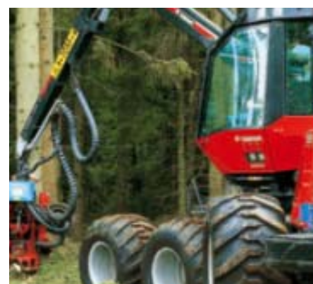
The Valmet harvester fells, delimits and cuts trees to size for a pre-determined purpose in less than one minute.
