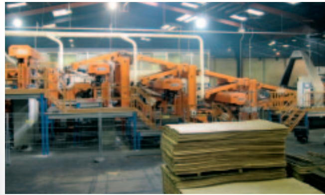
The veneer patching line delivered to France applies Mecano's machine vision technology.
