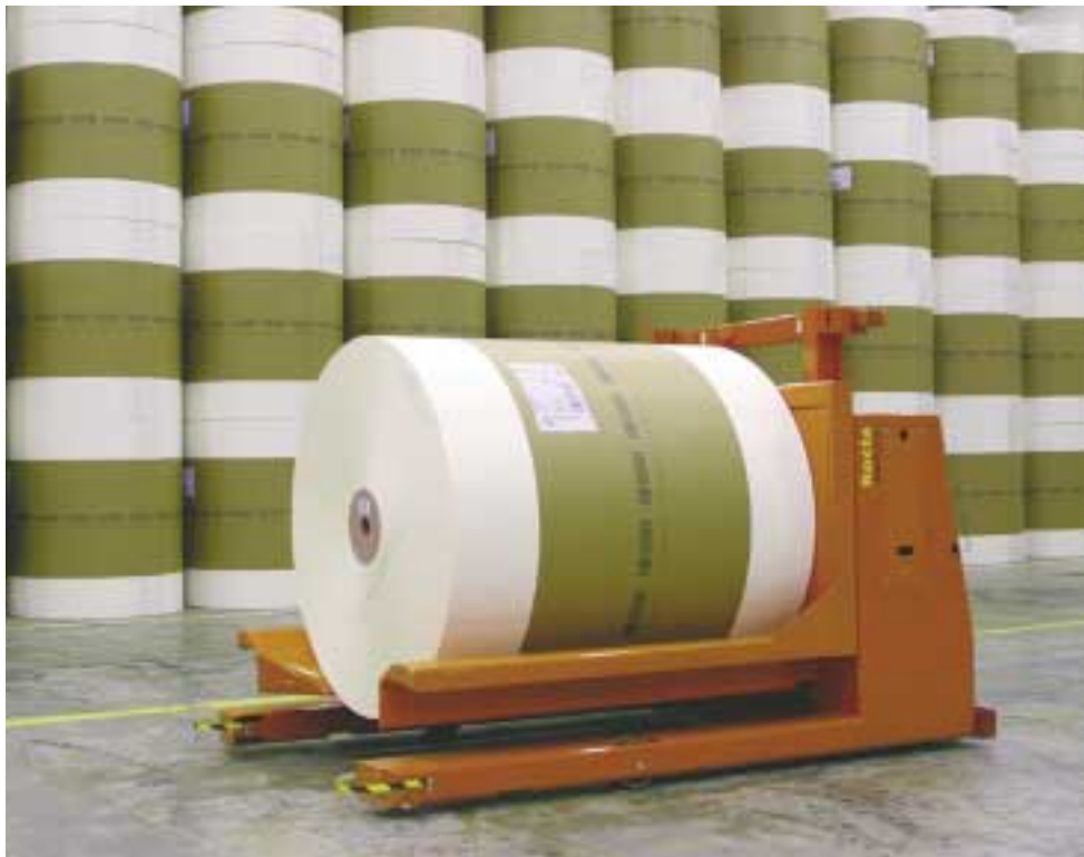
Rocla Robotruck is the global market leader for paper industry heavy-duty AGV-systems.
