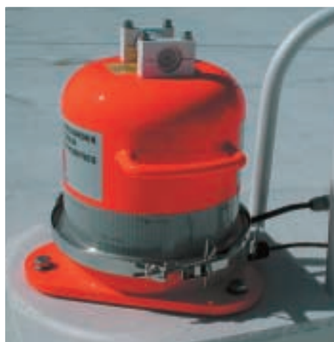
VDR stands for Voyage Data Recorder and is similar to the “black box” on an aircraft.
