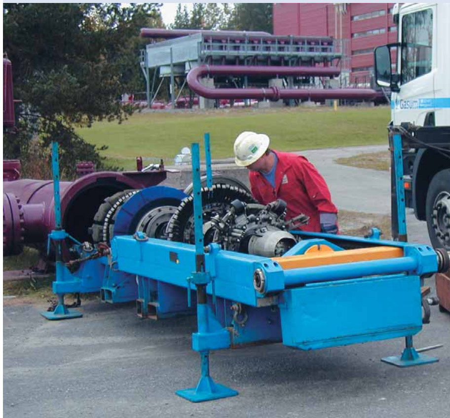
Lawrence Ling of PII-Pipetronix sends a smart pig off on its inspection journey at the Imatra reception station.
