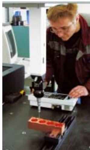
*A coordinate measuring machine is one of the tools used for the quality assurance of machined products.*
