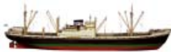
MS Fintrader (I) , (1951–1970) 6,435 DWT, 12 passenger berths, speed 15 knots. Built in the Netherlands.
