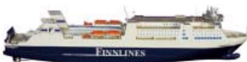
MS Finnclipper (II) , (1999–) Ro-pax vessel 2,500 lane metres, 440 passenger berths, speed 21 knots. Built in Spain.
