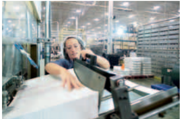
Final touches to a stack of printed cartonboard sidewalls before they are formed into ice cream containers in a Huhtamaki Systems forming machine.
