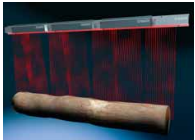
Smart Scan measures and centralizes the block with laser technology.
