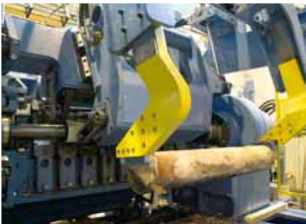
Smart Peel improves the veneer recovery and quality and the efficiency of production.
