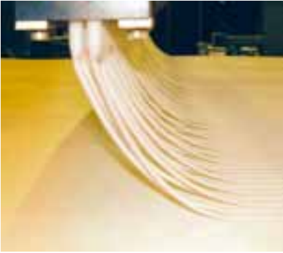
Foam gluing substantially reduces glue consumption.
