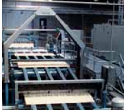
The machine vision system grades the veneers efficiently and accurately.
